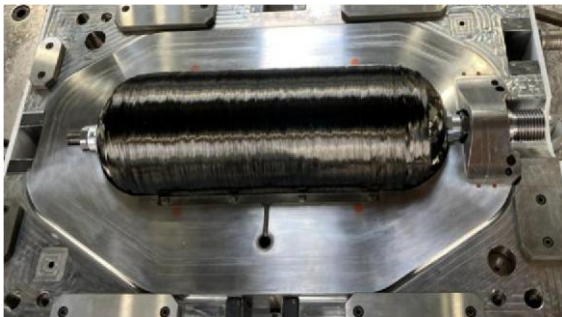
Figure 1 (Left): Dry carbon fiber wound onto a PA6 liner inside the mold before T-RTM process.
