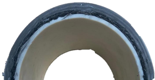
Figure 1 (Left): Dry carbon fiber wound onto a PA6 liner inside the mold before T-RTM process.
